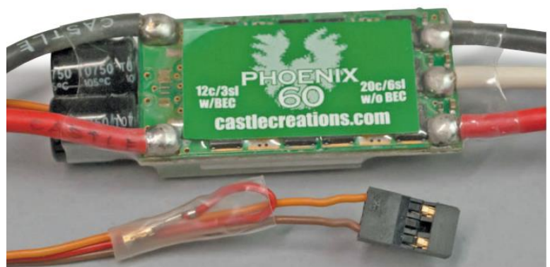
The BEC on this ESC has been disabled by removing the red pin from the receiver plug.
