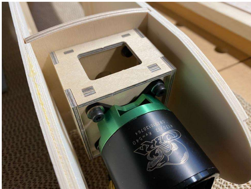
Huey Nguyen is building a BTE Venture 60, kitted by Bruce Tharpe, who designed some incredible kits while employed at SIG including the 1/3-scale Spacewalker, the Four Star 40 and 120 and others. The Venture 60 kit does not include the motor mount. Huey designed his own using CAD software and cut it using his home CNC machine. Bruce Tharpe was so impressed with Huey's design that he asked Huey to share the design files with him! What an incredible acknowledgement to Huey's skills!
